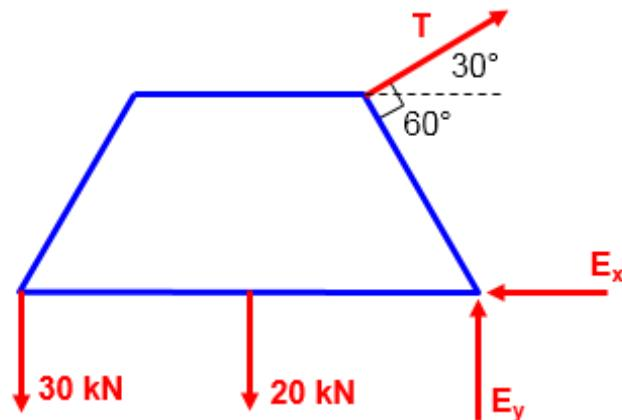
$$\begin{aligned}\sum M_E = 0 &\Leftrightarrow (-T \times 5) + (20 \times 5) + (30 \times 10) = 0 \\ \Rightarrow T &= 80 \text{ kN}\end{aligned}$$
