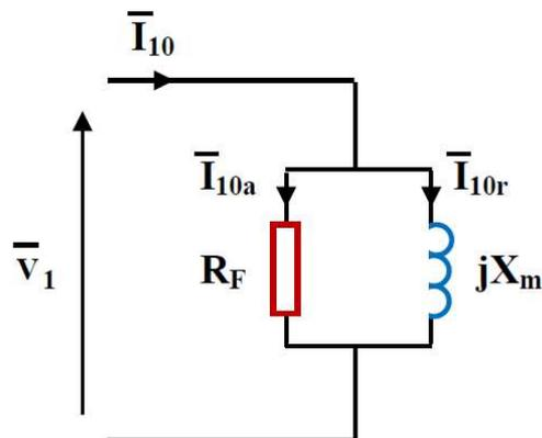
$$P_{10} = \frac{3V_1^2}{R_F} = \frac{U_1^2}{R_F} \Rightarrow R_F = 40.3 \text{ k}\Omega$$
