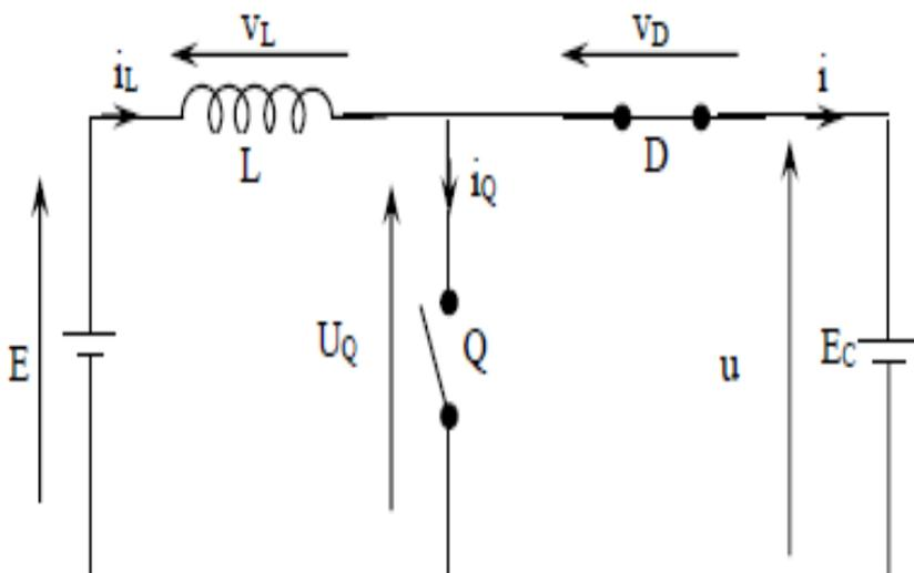
$$\begin{aligned} \text{On a : } U_Q &= E_C \\ v_D &= 0 \\ i_Q &= 0 \\ i_D &= i_L \\ \text{et } v_L &= E - E_C = L \frac{di_L(t)}{dt} \end{aligned}$$
