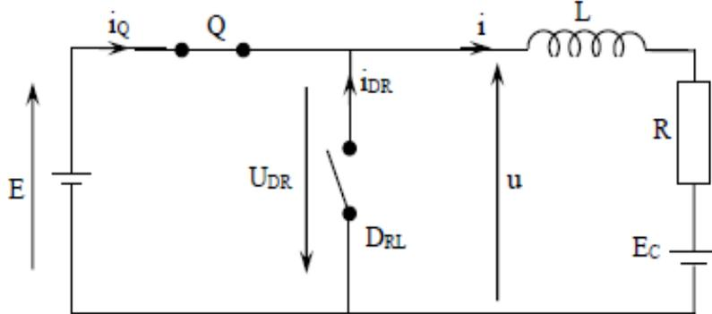
$$\begin{aligned} \text{On a : } U_{DR} &= -E \\ u &= E \\ i_Q &= i \\ i_{DR} &= 0 \\ \text{et } E &= E_c + Ri(t) + L \frac{di(t)}{dt} \end{aligned}$$
