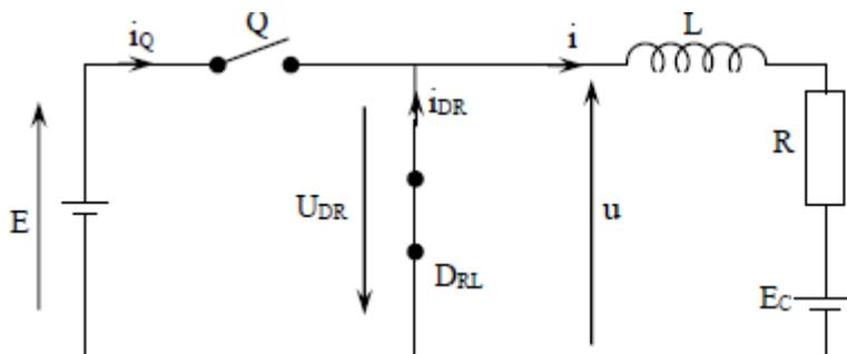
$$\begin{aligned} \text{On a : } U_{DR} &= 0 \\ u &= 0 \\ i_Q &= 0 \\ i_{DR} &= i \\ \text{et } 0 &= E_c + L \frac{di(t)}{dt} \end{aligned}$$
