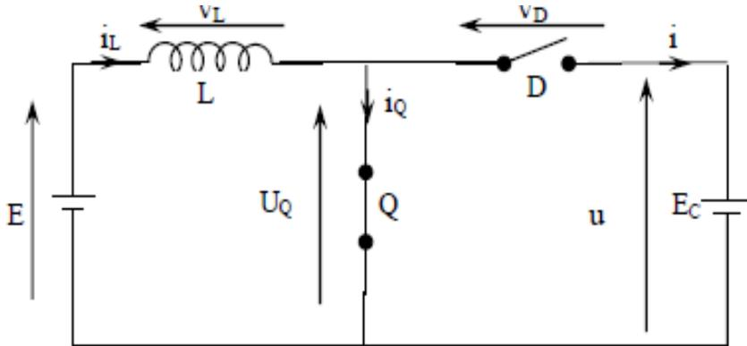
$$\begin{aligned} \text{On a : } U_Q &= 0 \\ v_D &= -E_C \\ i_Q &= i_L \\ i_D &= 0 \\ \text{et } E &= v_L = L \frac{di_L(t)}{dt} \end{aligned}$$
