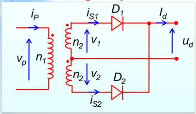
$$v_1 = V_m \sin(\omega t) = -v_2$$
