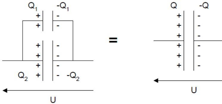
$$\begin{aligned} Q_1 &= C_1 U \\ Q_2 &= C_2 U \\ Q &= C_{\text{éq}} U \end{aligned}$$
